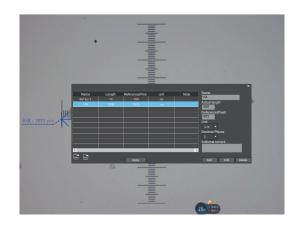
Step 4: Enter a name in the calibration table, such as 10X. In the calibration table, enter the actual length that just drawn on the micrometer, for example, the sample figure is drawn 100 DV, that is, 1mm, or 1000µm, then enter the "actual length" box to fill in the specified 1000, "unit" select "µm". Then click "Add" to add this calibration value to the calibration table to be used. Add the calibration value for other objectives of different magnifications in this way.
