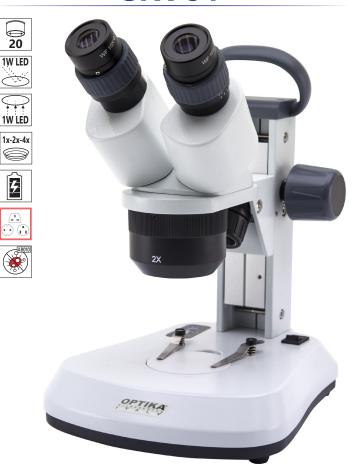
Cordless binocular stereomicroscope ideal for students, schools and amateurs to dissect and discover mainly biology and materials science in 3D, with turnable objective (1x-2x-4x), FN 20 eyepieces, precision fixed arm with handle and 1 W LED transmitted / incident illumination with comfortable touch control and rechargeable batteries. Slim and easy to carry, it is equipped with long lasting LED illumination to provide over 20 years of use
