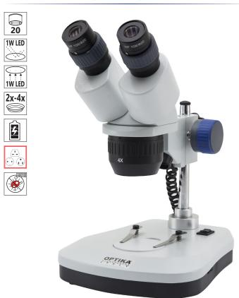
Cordless binocular stereomicroscope ideal for students, schools and amateurs to dissect and discover mainly biology and materials science in 3D, with turnable objective (2x-4x), FN 20 eyepieces, pillar stand and 1 W LED transmitted / incident illumination with rechargeable batteries. Slim and easy to carry, it is equipped with long lasting LED illumination to provide over 20 years of use
