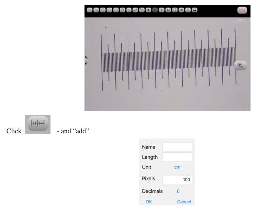
Place the calibration scale within the microscope's field of view.
