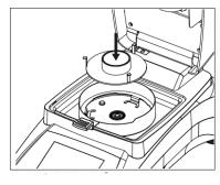
Press the **Start** to initiate the temperature adjustment process. Follow the screen prompts throughout the process.
