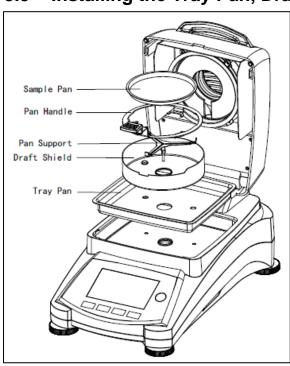
Lift the cover straight up and Install the tray pan in the base of the heating chamber.
