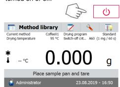
The **Moisture Analyzer** turns on automatically when connected to a power source. An internal diagnostic test is performed; the display lights and the Home screen appears followed by the initial display.
