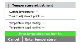
This is a two-point adjustment (100°C and 160°C). The dryer unit now heats to the second temperature (160°C). Adjustment of the temperature is defined by two points. Proceed exactly as you did for the first temperature. After you have set the display to agree with the thermometer, then press the **Enter** button.
