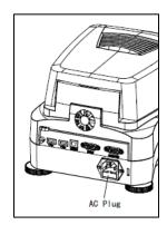
Connect the power cord to the power supply socket located at the rear of the Moisture Analyzer and to the power supply outlet. The Moisture Analyzer becomes operational as soon as power is applied.
